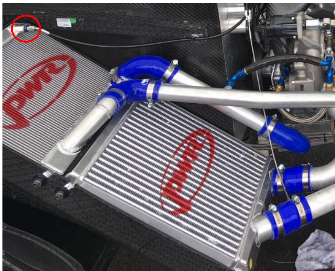
Figure 2: (Radiator Bleed Port – left side - typical)
