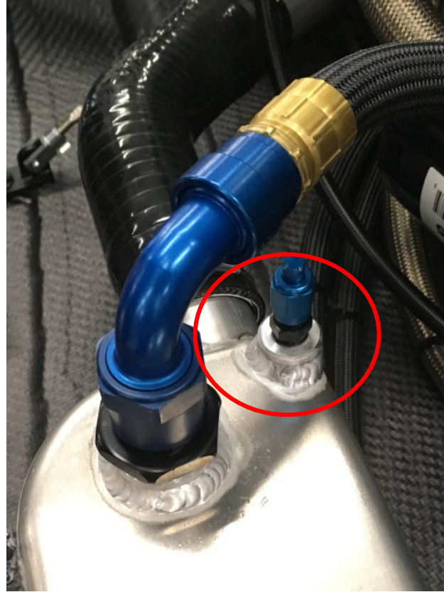
Figure 4: (Radiator Bleed Port – right side - typical)
