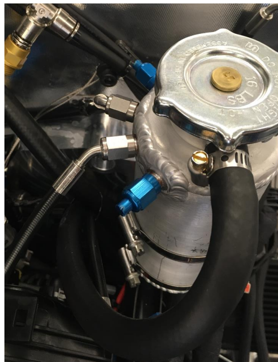
Figure 6: (Cylinder Head Port – depicted here with a constant bleed line directly behind the water temperature sensor)
