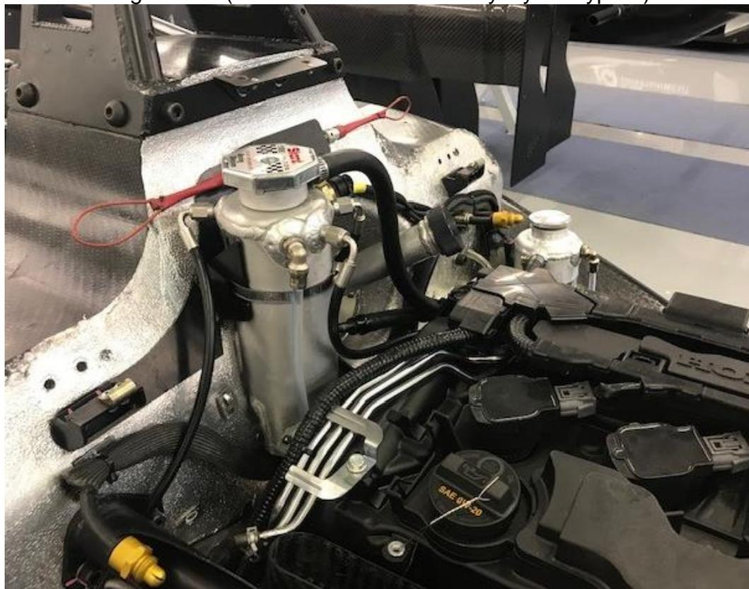
Figure 6: (Cylinder Head Port – depicted here with a constant bleed line directly behind the water temperature sensor)
