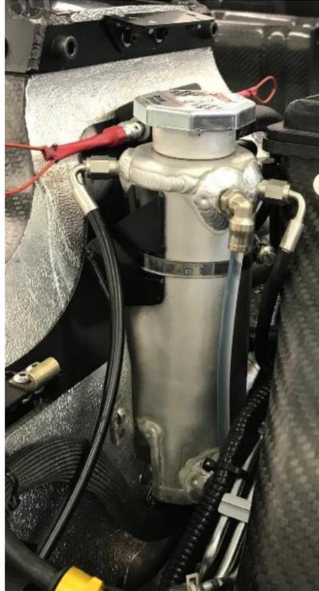
Figure 5.2: (Recovery Tank - typical)
