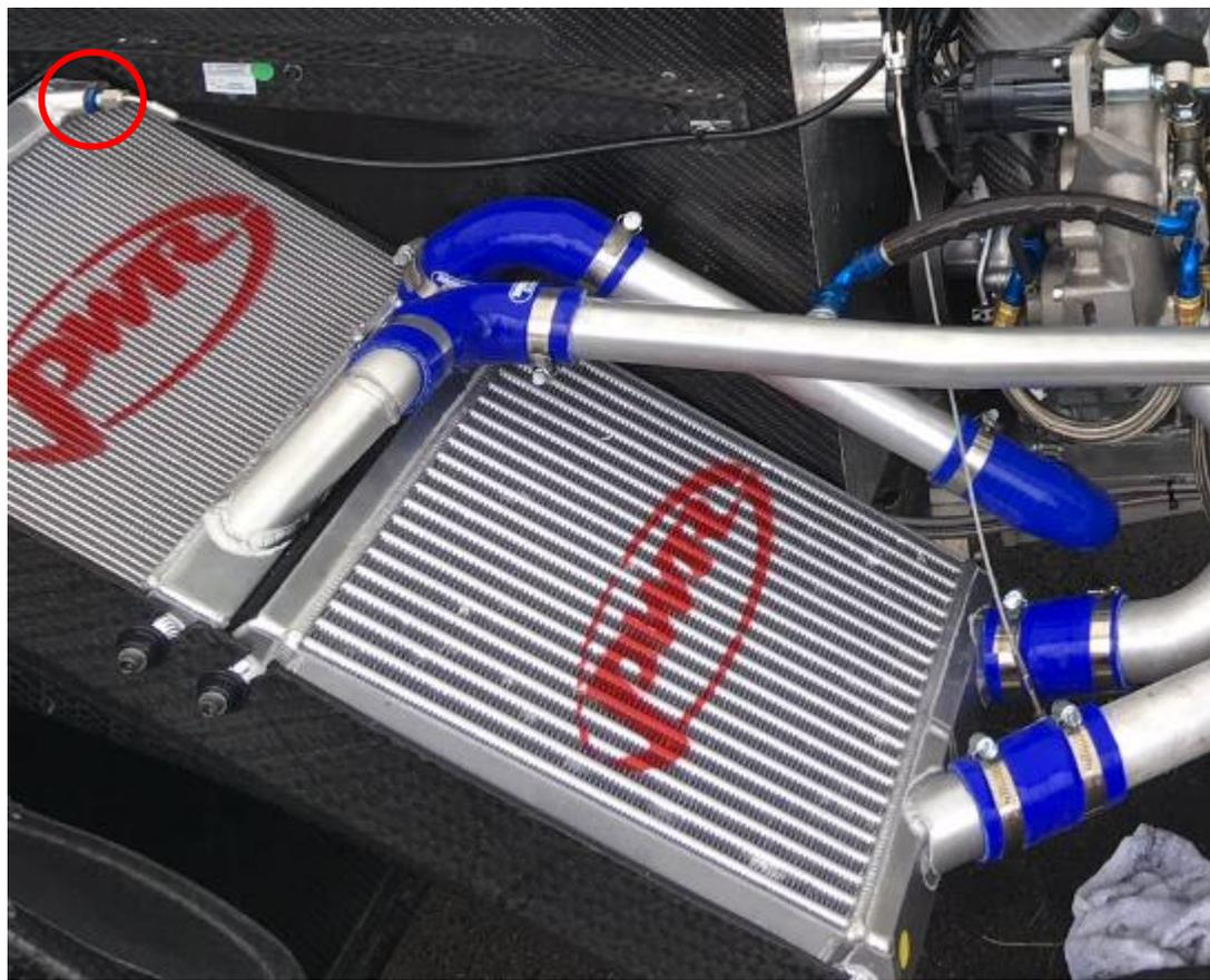
Figure 3: (oil cooler Bleed Port - typical) – this port to remain capped.
