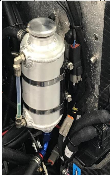
Figure 5.3: (Header Tank and recovery layout- typical)
