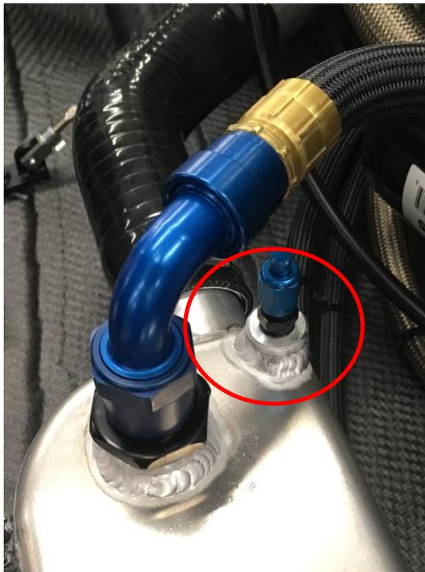
Figure 4: (Radiator Bleed Port – right side - typical)
